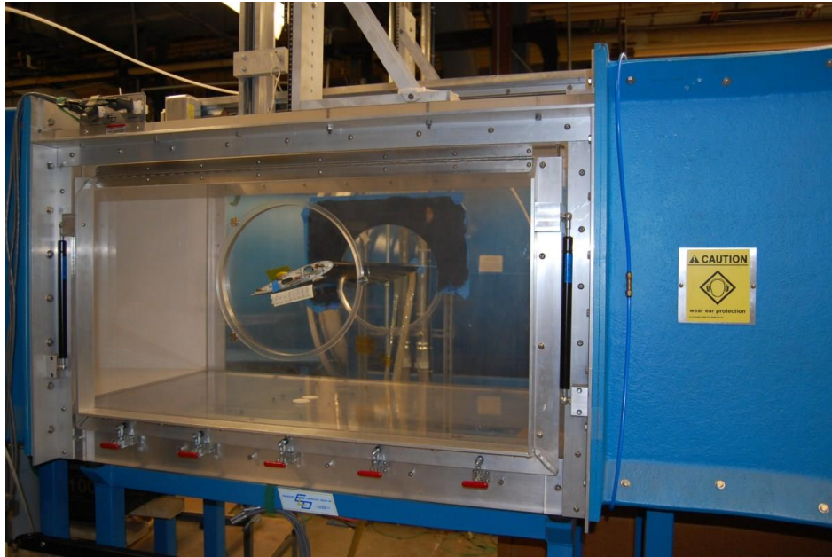
Figure 1: Airfoil mounted in test section.
