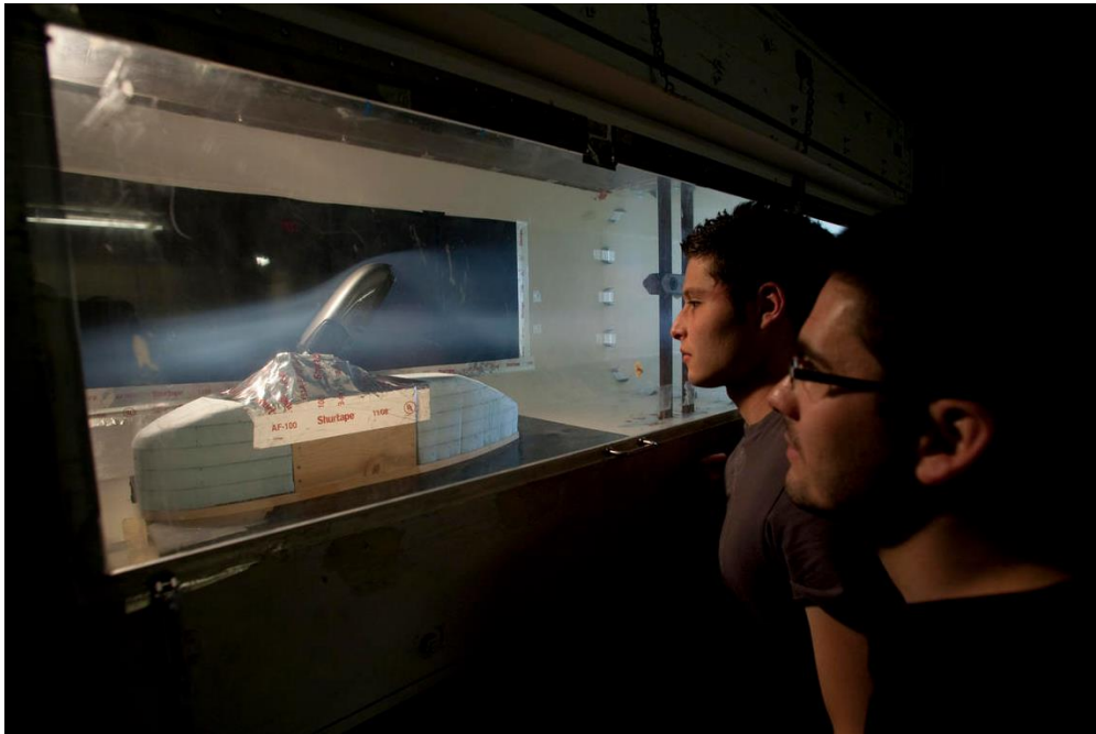
Figure 1: A side-view mirror model is being tested using smoke visualization.
